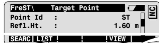
To define a list of the target points and the measurement sequence.
