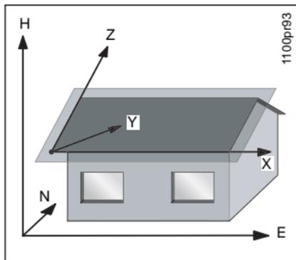
A tilted plane is defined by 3 or more points. The Z-axis is determined by the steepest grade, the Y-axis is the normal vector. X is perpendicular to both and horizontal.
