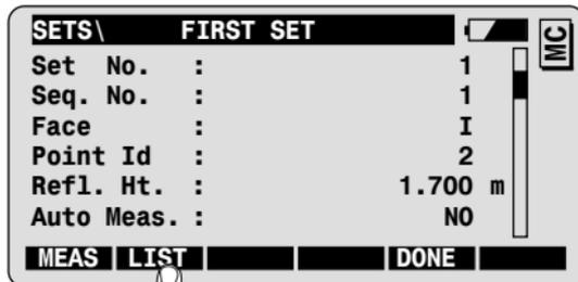
To define a list of Target points and the measurement sequence.
