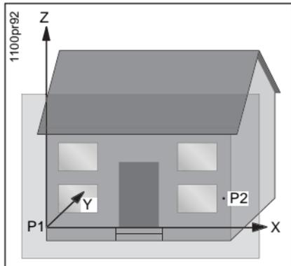
A vertical plane is defined by 2 points. The X-axis goes through P1 and to the right (as seen from the station). It is horizontal.
