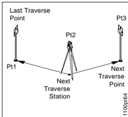
The instrument has been set up on the next traverse station.
