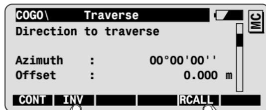
To start the inverse function to determine azimuth.
