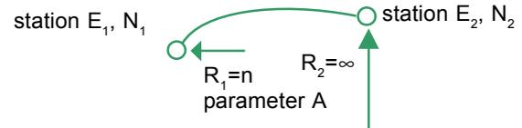
**Curve in** - spiral transition from larger to smaller radius curve.
