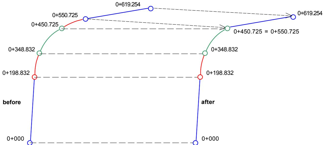
Due to removing a constituting element, the sequence of stationing misses some values. If this is the case, a **gap equation** (forward station equation) is required. The station equation is of the form:
