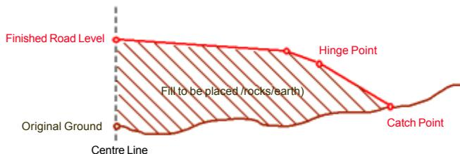
**L.End Slp <%>** - A slope at the leftmost point of the cross section can be defined in percent. If the design surface is falling to the left, the slope is a positive value (see chapter "Design Elements").
