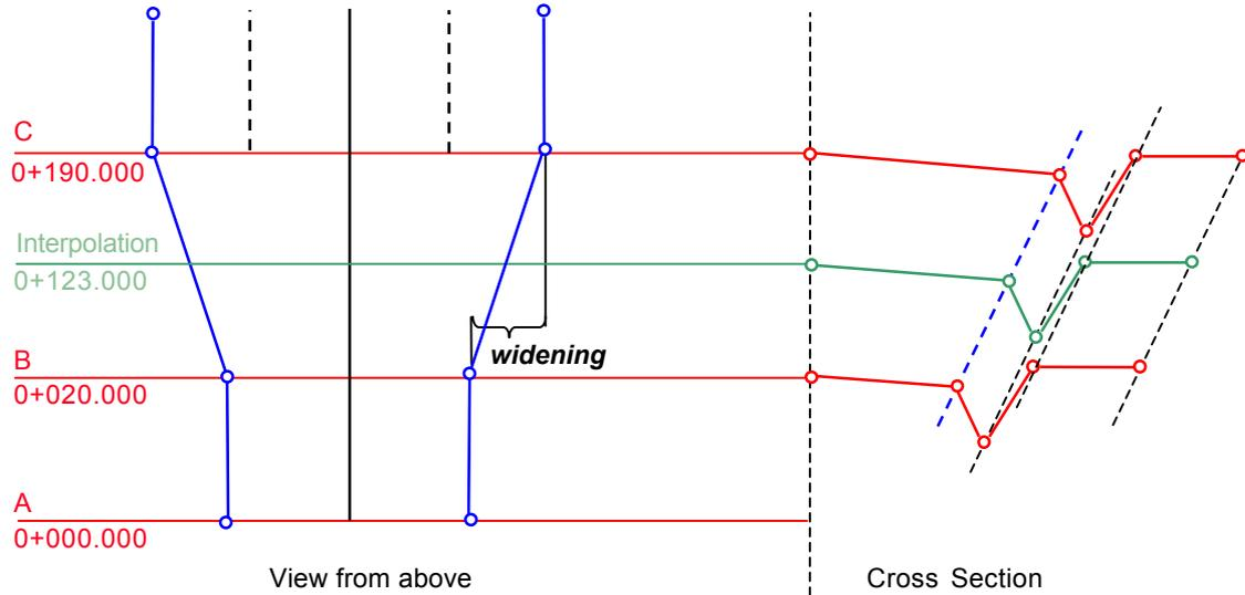
**Superelevation** - modification of the normal pavement cross slope. Intended to increase comfort and safety at speed.
