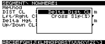
For entering the segment information, select between method **Delta Dist CL** and **Cross Slp<%>**. Depending on the selected method, the input fields change. Both methods are described in the following section.
