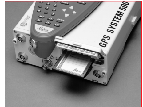
Inserting the PC Card
